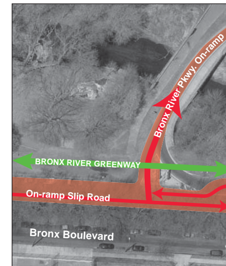
Figure 4: Proposed normalization of on-ramp intersection
