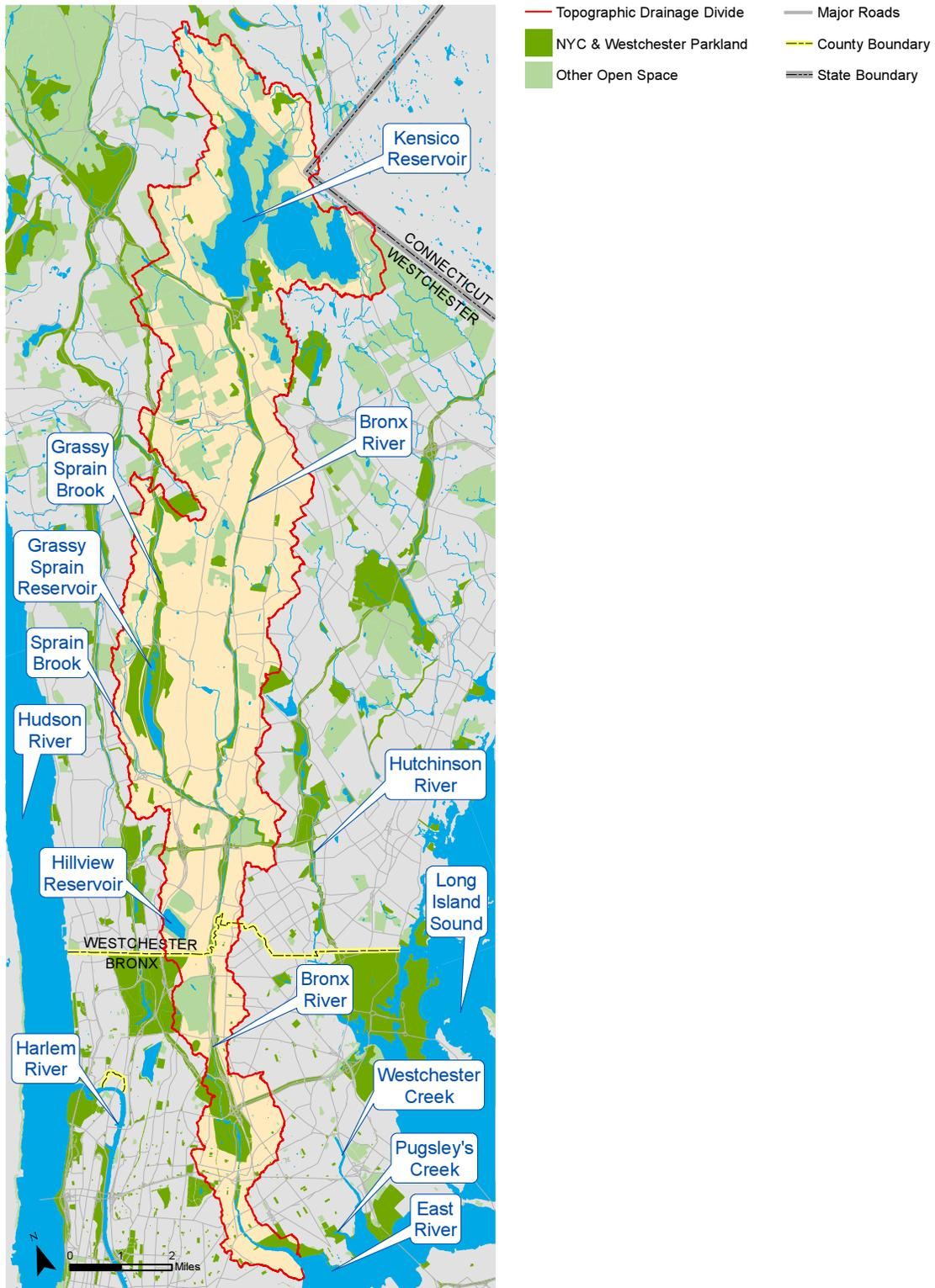
The topographic drainage divide (red line) encompasses the 56 square mile Bronx River watershed, or region of land where water from rain or snowmelt drains downhill into the river. The drainage basin includes both the streams and rivers that convey the water as well as the land surfaces from which water drains into those channels.
